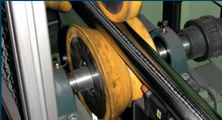
Guide and pressure rolls with exchangeable cores
